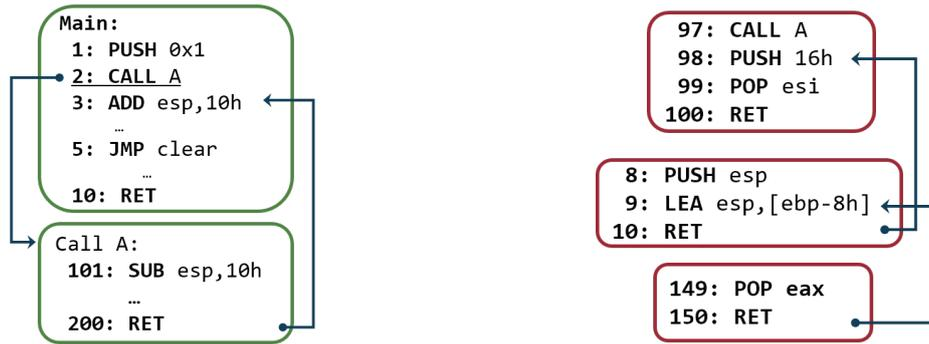
(a) In normal function call, return addresses target valid (b) In ROP attack, return address is valid or invalid
