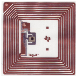
Figure 1.1: A Typical Passive-RFID Tag (Source: Texas Instruments: Tag-it TM )
