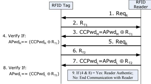
**Fig. 1.** Security Weakness of EPCglobal Class 1 Gen 2 UHF RFID Protocol
