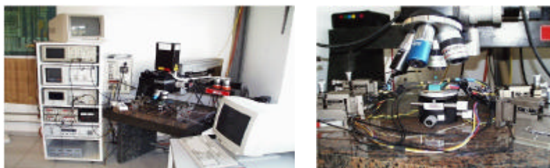
Access to CPU Bus via Laser Depassivation and Microprobing
