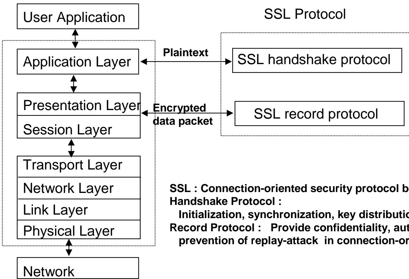
**SSL : Connection-oriented security protocol between C/S**
