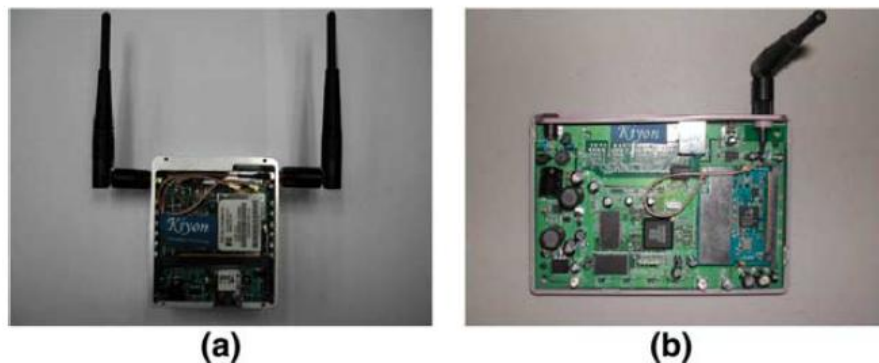
Figure 2.1: Examples of mesh routers based on different embedded systems: (a) PowerPC (b) Advanced RISC Machines (ARM) [8]
