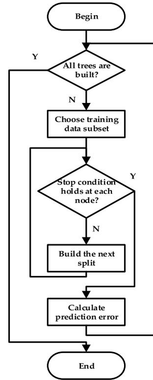
Fig. 6. Flowchart of Step III ensemble.
