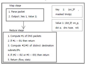
Fig.2 Design of Module 2 in Hadoop framework.
