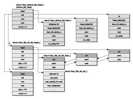
Fig. 6 The structure of File & Directory on Micro-Kernel
