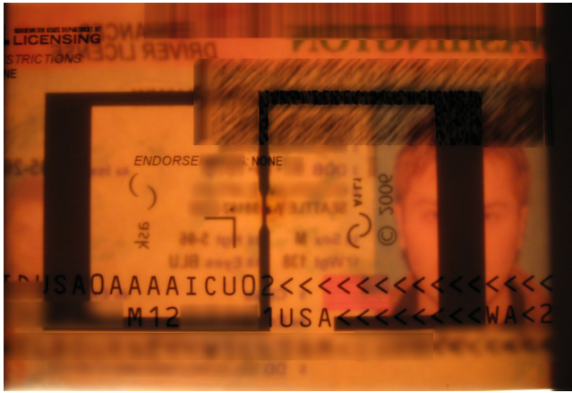
Figure 1: The antenna inside a Washington State Enhanced Drivers License. Certain personally-identifiable information has been obscured.
