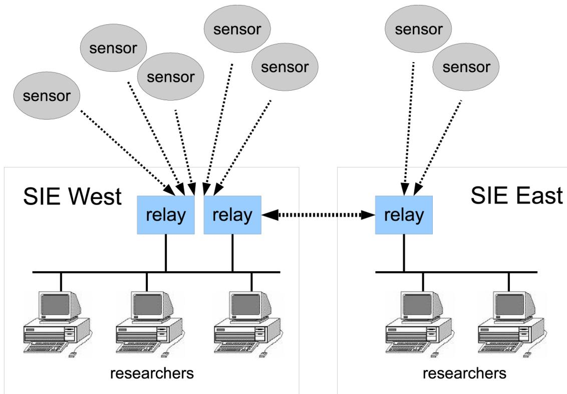
Real-time broadcast ensures that multiple replay switches see identical traffic
